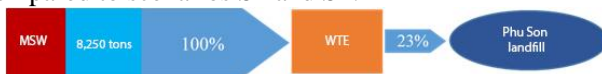
Figure 4.8. Scenario 3 (S3) – All MSW is taken to Phu Son waste to energy plant and treated by incinerating to recovery energy
